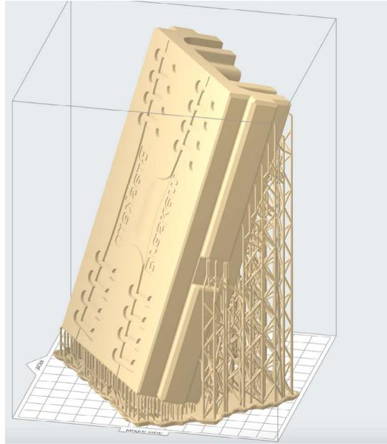
*The final CAD file of mold loaded into Formlabs PreForm print preparation software. The part was printed tilted with supports. Smaller molds can also be printed directly on the build platform to minimize post processing time.*
