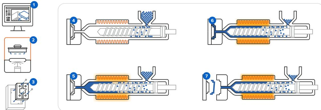
1 Mold design 2 Mold 3D printing 3 Mold assembly 4 Mold clamping 5 Injection 6 Cooling 7 Demolding
