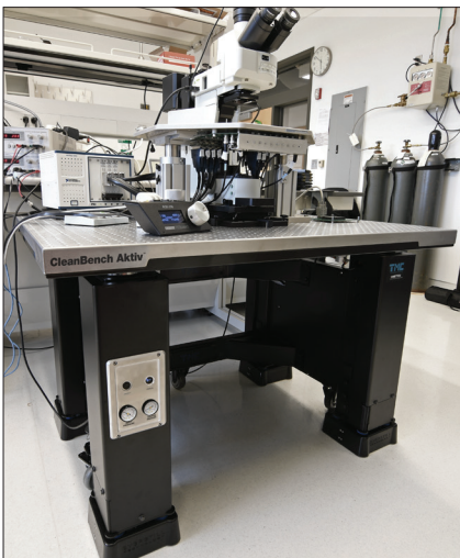
CleanBench Aktiv table supporting an optical microscope for a life-science research application (image courtesy of Harvard University)
